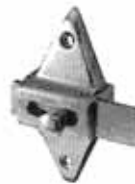
SLIDE BOLT ASSEMBLY 2-3/4" Bet. Screws 9/16" Bar to Door Clearance Part No. 9F0302
