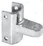
TOP HINGE 1-1/2" Bet. Screws Part No. 9C3503 A = 1-7/16"
